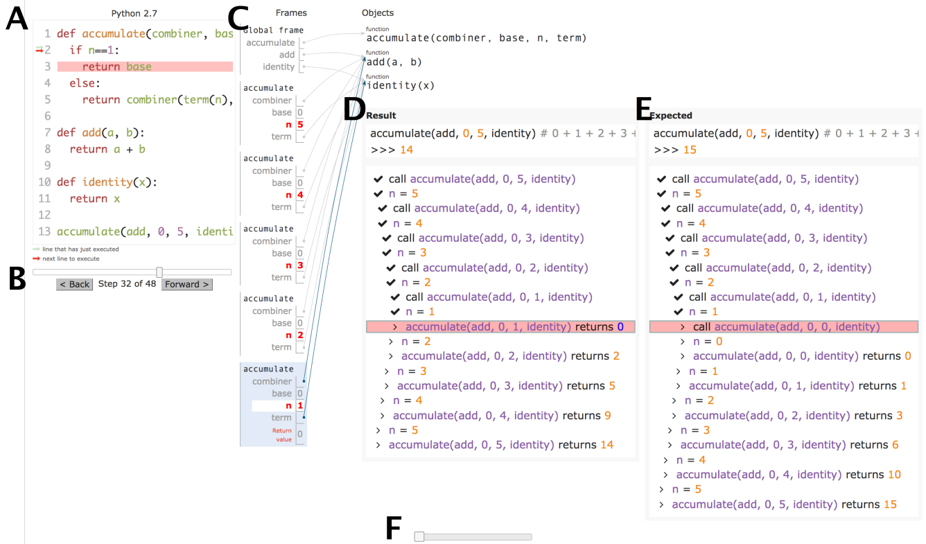
Fig. 2. The system interface consists of a code editor (A), a visual debugger (B-C), extracted code traces (D-E), and a slider for interactive abstraction (F).
